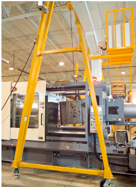
Caption: Thogus Products Companies first tool inserted in its new 720 ton machine.
